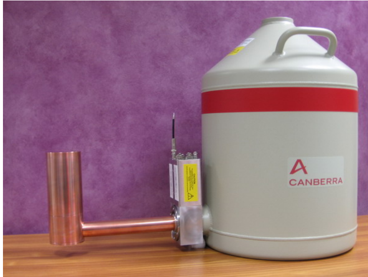
Modified electrode 50x50 ULB detector
