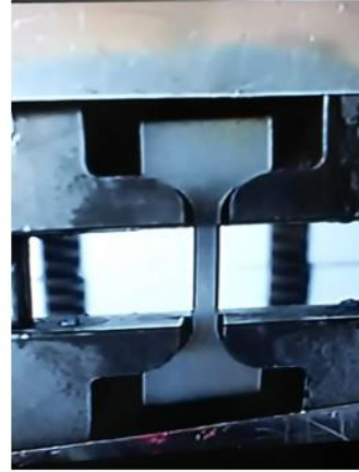
Figure 6 : (Left) Ideal stress-strain curve obtained with tensile testing. (Right) Tensile test at Pacific Northwest National Laboratory (PNNL). By tensioning a dogbone-shaped specimen, the relationship between elongation relative to the original length (strain) and load per unit cross section (stress) is obtained, which provides mechanical properties required for vacuum window design.
