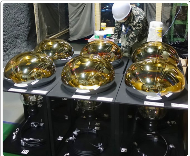
The new photosensors developed for Hyper-K Provided by: The University of Tokyo, Institute for Cosmic Ray Research, Kamioka Observatory
