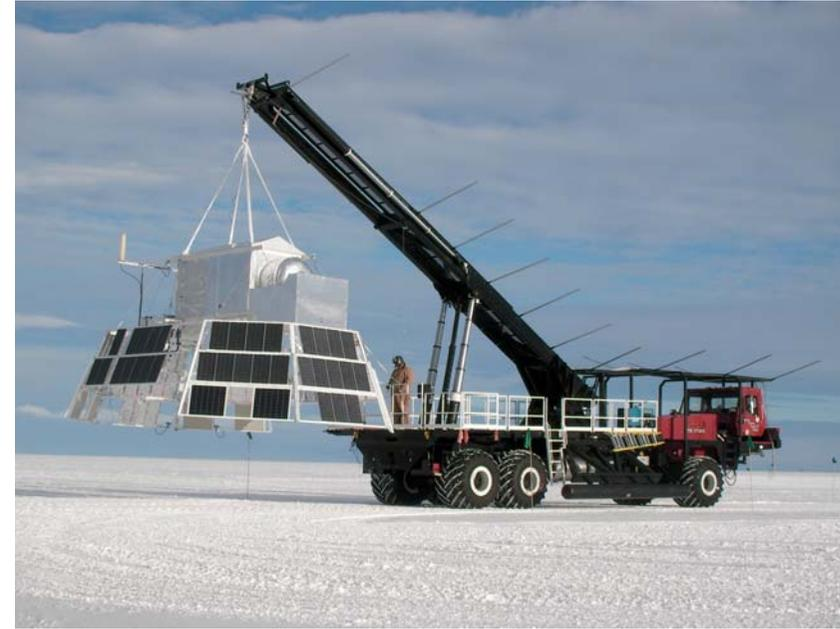
Hang test prior to flight (11/27) was successfully done
