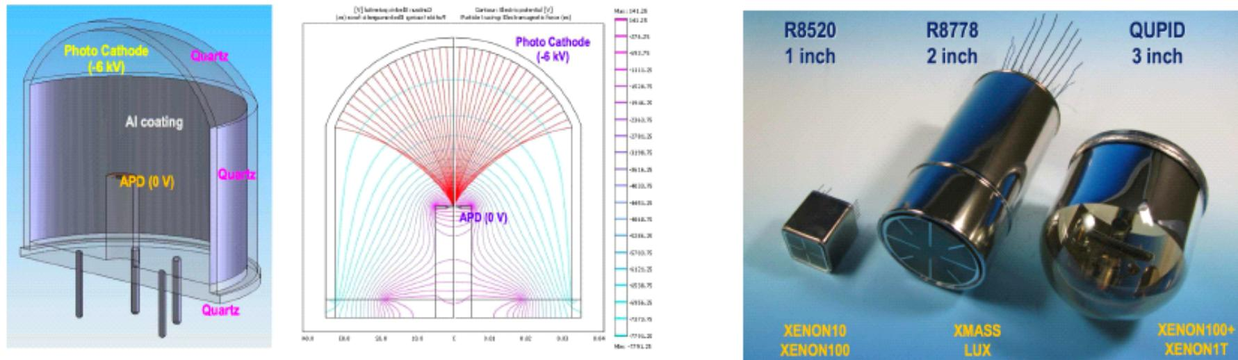
Figure 8: Left: Structure of a QUPID, made of pure Quartz with a 3 mm diameter APD at its center. Center: Simulation of electron trajectories, showing that all photoelectrons from the photocathode are well focused onto the APD. Right: Comparison of R8520 (used in XENON10/100), R8778 (used in LUX), and QUPID.
