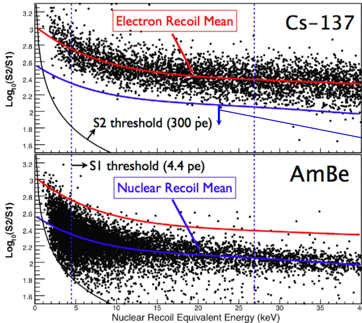
*~ 99.5 % gamma events are rejected below the nuclear recoil mean*
