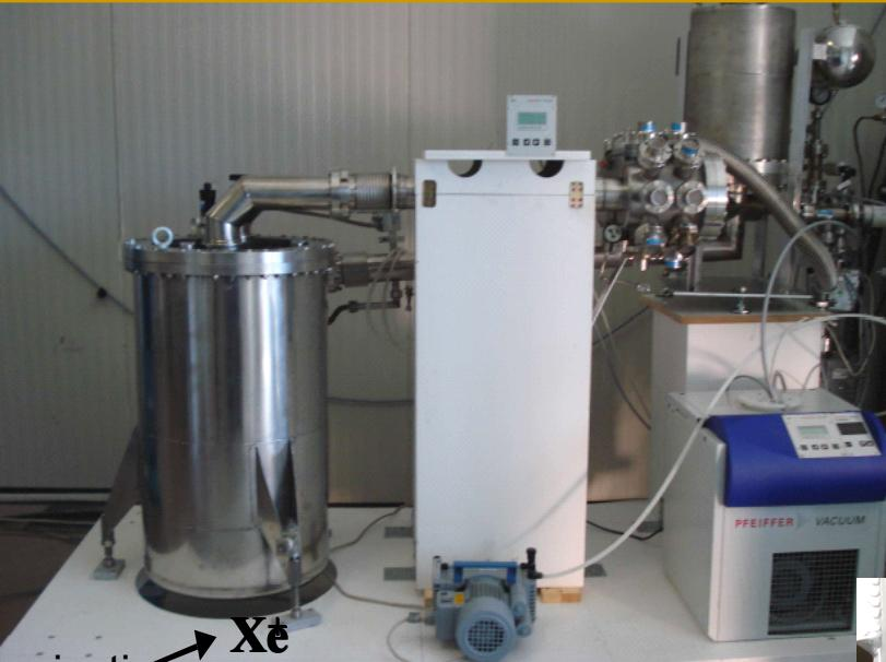
Pulse Tube Refrigerator (160 W) for Xe liquefaction and gas recirculation
