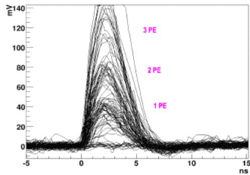
Figure 9: Typical waveforms taken with a QUPID. The three waveform bands at 40, 80, and 120 mV correspond to 1, 2 and, 3 photoelectrons.
