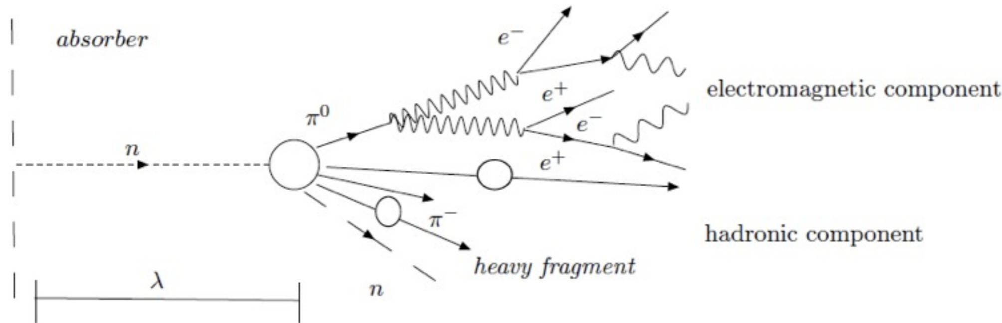
A calorimeter typically responds differently to the different components of the shower
