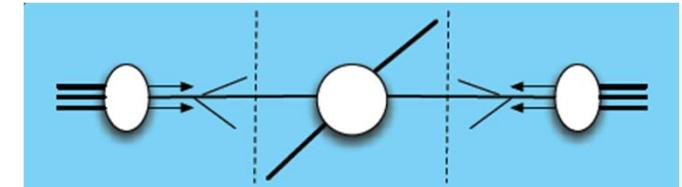
$$\sigma = \sum_{pdf} \int dx_i dx_j [f_i(x_i) f_j(x_j)] \times \Delta\sigma(q_i q_j \rightarrow X; x_i, x_j)$$
