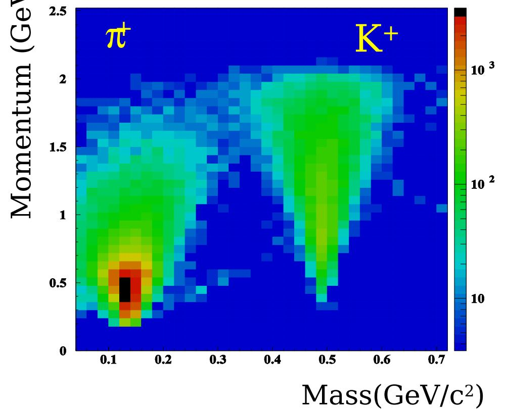
$$\sigma_{\text{Mass}} = 30 \text{ MeV}/c^2 (\text{typ.}) \text{ for } 1 \text{ GeV}/c \text{ Kaon}$$
