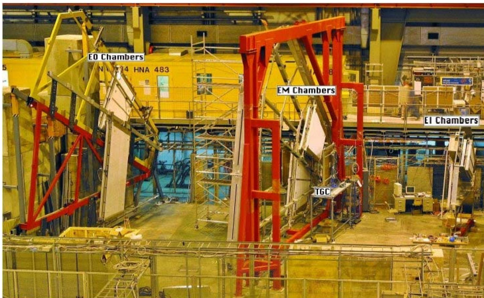
Shown in this picture is the end-cap set-up, it is preceded in the beam line by a barrel sector
