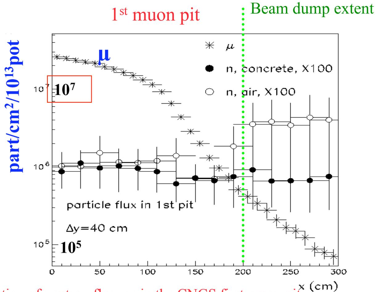
An updated calculation of neutron fluence in the CNGS first muon pit,
