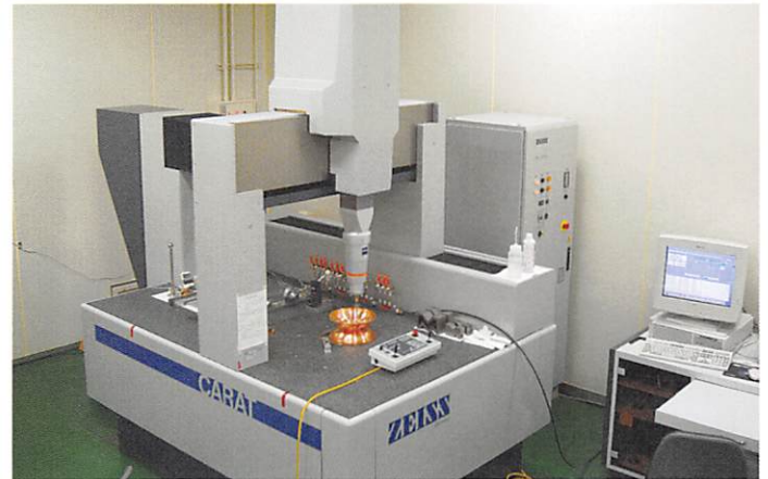
Precise dimension measurement by \mu\text{m} order using 3D coordinate measuring equipment
