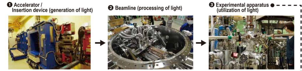
The development of insertion device technologies such as undulators has made it possible to obtain high-brightness, polarization-controlled light (photo: undulator at BL-2).
