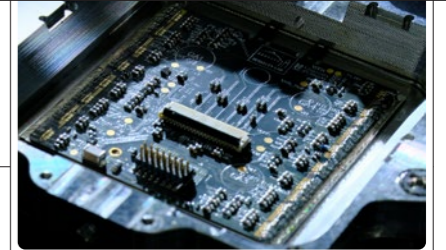
Pixel semiconductor detector modules in the inner tracker for the HL-LHC experiment will measure charged particle trajectories with improved precision.
