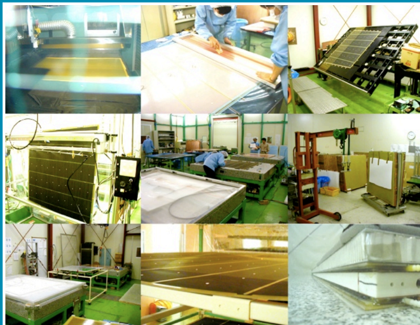
Tanaka and his team designed and built the TGC production line which successfully produced 1,200 TGCs on schedule. (Upper row, left to right) Graphite spraying, framing, and wire winding on rotary. (Middle row left to right) Cleaning, making a singlet module, and sandwiching a paper honeycomb with two TGCs. (Lower row, left to right) making a doublet module, an image of singlet module, and an image of doublet module.
