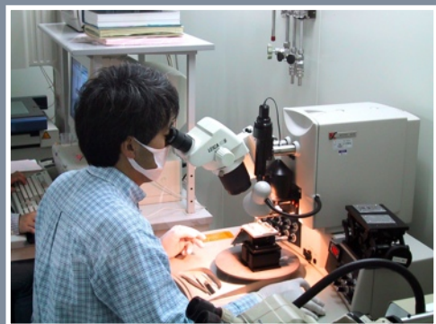
Kohriki manually bond thousands of wires on the prototype flexible board.
