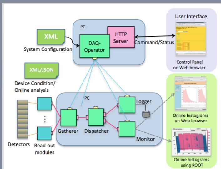
The key technology of DAQ-Middleware is the web technology. Upon reception of a command from the control panel on a web browser, the DAQ-Operator searches an XML database for the list of required DAQ-components, and generates the components. The gatherer and monitor components in the readout module are the only software components that are detector-specific.
