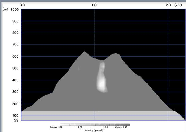
An image of Mt. Iwodake obtained by cosmic-ray muon radiography. Dark area represents high-density region, and light area represents low-density region. (Image courtesy of the Earthquake Research Institute at the University of Tokyo)
