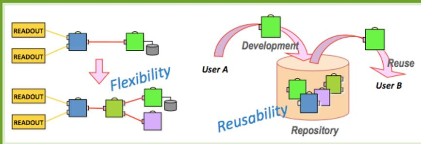
The advantage of the DAQ-Middleware is the flexibility of component configuration, and reusability of already developed components.
