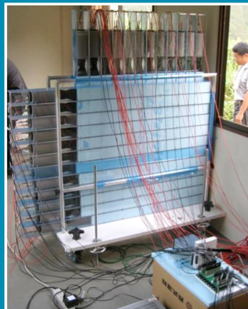
Muon counter (center) and readout module (lower right). The low-power SiTCP hardware enabled solar-powered readout electronics for cosmic-ray muon radiography to probe volcano internal structure in real time.
