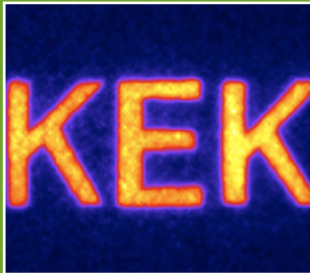
A GEM detector can also detect photons. This is a hard X-ray image of a plate punched with the letters 'KEK'.
