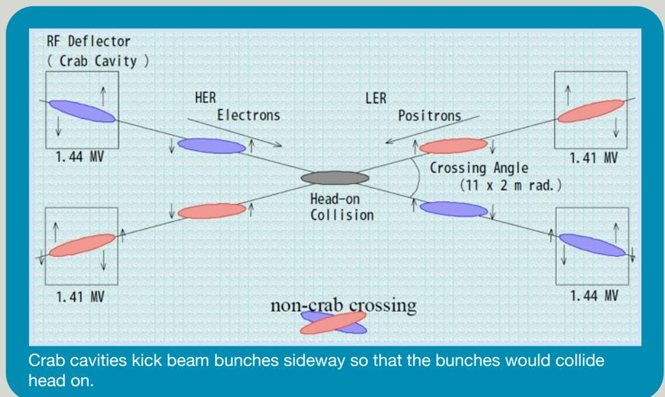
Crab cavities kick beam bunches sideways so that the bunches would collide head on.
