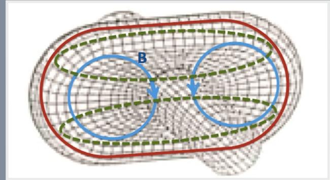
The oval-shaped crab cavity creates two-loop magnetic field (blue) inside to kick bunches sideways. It is called crab mode. Unwanted modes, accelerating mode (red) and vertical polarization mode (green), are also excited.
