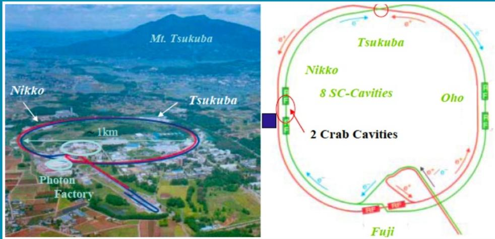
Two superconducting crab cavities were installed in the KEKB accelerator ring at KEK.
