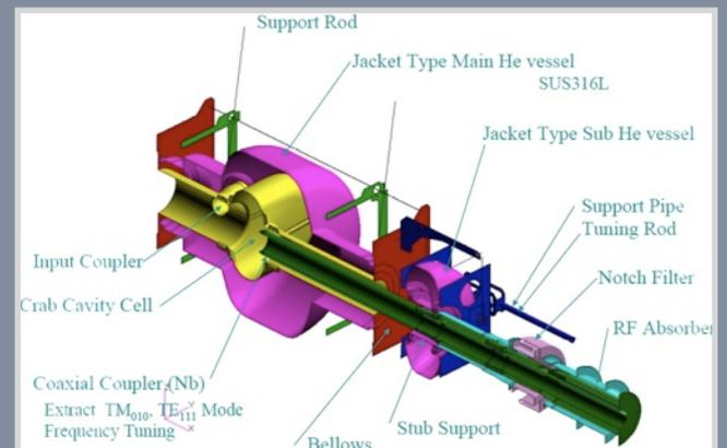
cavity, 1.5 meters long and 1 meter wide, was a challenge at the time of fabrication and when trying to rotate the cavity during electro polishing and rinsing.
