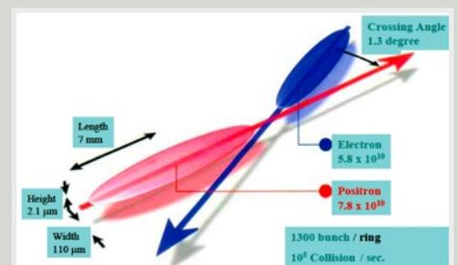
KEKB's beams of electrons and positrons make a finite angle when they cross.
