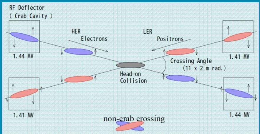
Crab cavities kick beam bunches sideways so that the bunches would collide head on.
