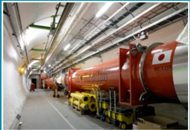
The final focus line. The quadrupole magnets embedded deep inside the cryomodules, which were produced by Fermilab, were designed and built by Prof. Akira Yamamoto at KEK.
