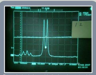
Two-peak signal observed in the laser beam stored in four-mirror optical cavity, showing that the incoming linearly polarized laser beam become circularly polarized as it circulates in the cavity. times per second. This is 10 times more than required to conduct the circular dichroism study of amino acids. Thus, this technology may bring about a revolution in the way we understand biological systems by helping to explain the broken symmetries in biochemistry.
