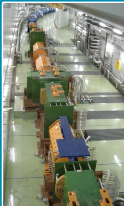
Superconducting magnets (blue magnets at the far end) guide the extracted beam of protons to T2K's final focusing section where the beam is focused to a proper size in normal conducting magnets (green and orange).
