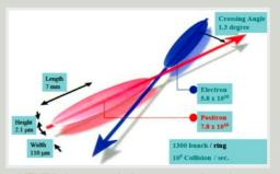
KEKB's beams of electrons and positrons make a finite angle when they cross.
