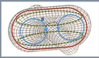
The oval-shaped crab cavity creates two-loop magnetic field (blue) inside to kick bunches sideway. It is called crab mode. Unwanted modes, accelerating mode (red) and vertical polarization mode (green), are also excited.
