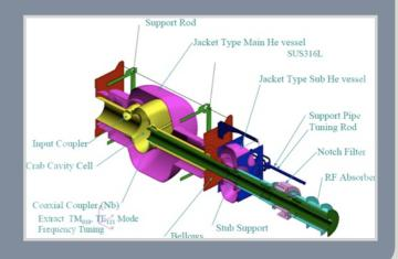
cavity, 1.5 meters long and 1 meter wide, was a challenge at the time of fabrication and when trying to rotate the cavity during electro polishing and rinsing.
