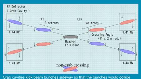
Crab cavities kick beam bunches sideway so that the bunches would collide head on.
