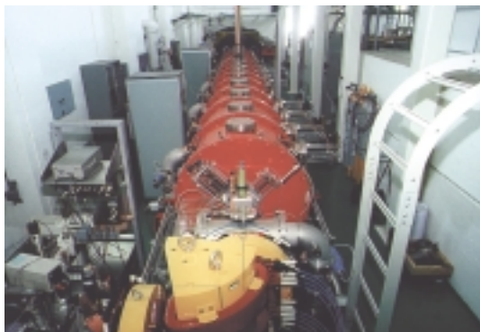
Heavy ion lineac constructed at the Tanashi Branch of KEK. This lineac will be used for acceleration of unstable nuclear beams at JHF.
